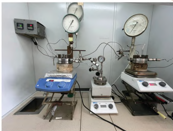
Fig. 1. Autoclave unit for the reaction of hydroalkoxycarbonylation of olefins
