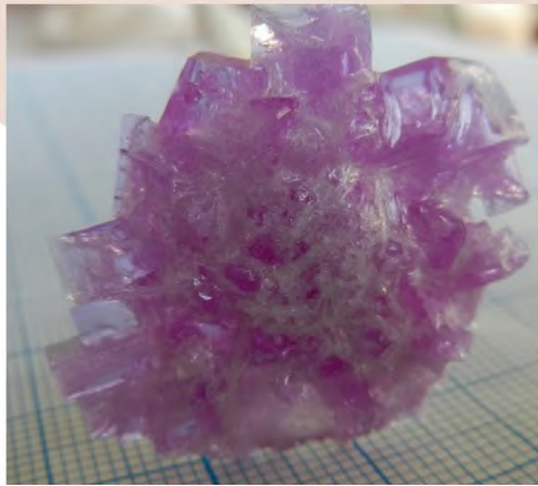
Figure 1. K_7CaNd_2(B_5O_{10})_3 crystal grown from K_2O-B_2O_3-CaF_2 flux
